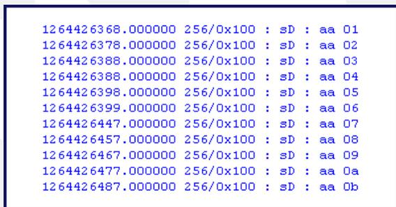
Particularly for commissioning and error analysis a precise time resolution of the received CAN messages at the network is necessary. The time represented by CAN-REport is influenced only by the used hardware. Time resolution up to 1 µs can be achieved by using CAN interface boards under the Linux operating
